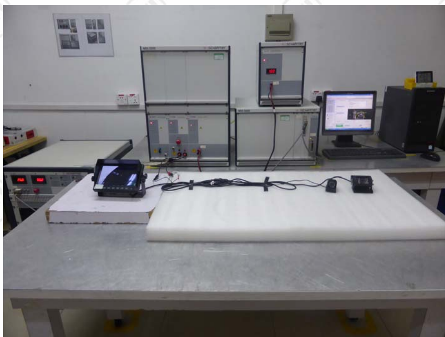
CONDUCTED TRANSIENT IMMUNITY TEST SETUP
