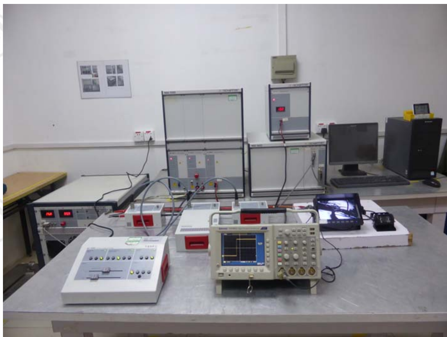
CONDUCTED TRANSIENT DISTURBANCES TEST SETUP
